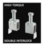
The bottom face of the 'U' has serrations, which grips the conductor firmly during tightening. The lips are drilled and threaded coaxially in a special machine to produce rolled threads for higher mechanical strength of threads which can take higher tightening torque.
