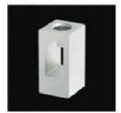
The clamping part in 'elimex' screw clamp is of special design, such that as the conductor clamping is achieved by tightening of screw, the top-portion bends elastically, so that screw threads are gripped to prevent loosening.
