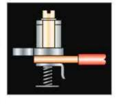
spring loaded terminals especially suitable for high vibration applications.
